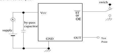
\*Current consumption under the disable function should be = GND.
