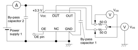
\* The lines from OUT and  $\overline{OUT}$  pin are same length.
