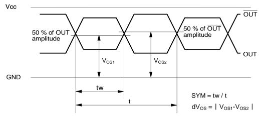
Differential output waveform (OUT –  $\overline{OUT}$ )
